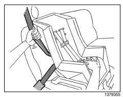
5) To tighten the belt, push down on the child restraint, pull the shoulder portion of the belt to tighten the lap portion of
